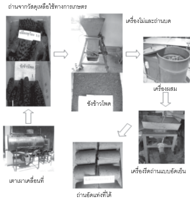
Figure 1 Compressed charcoal production Process.
