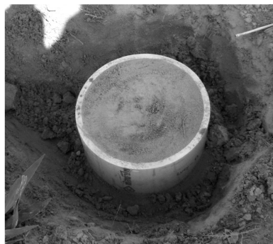
Figure 2 Soil sample collecting for evaporation method.
