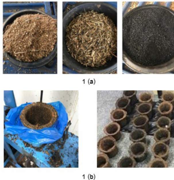
Figure 1 (a) Raw materials from decreasing process. (b) Bio-materials pot after forming by hydraulic machine and showing in each formula.
