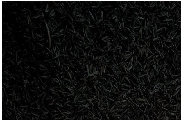
Figure 2 Characteristic of husk from combustion section of compressing machine, speed motor of 30 rpm
