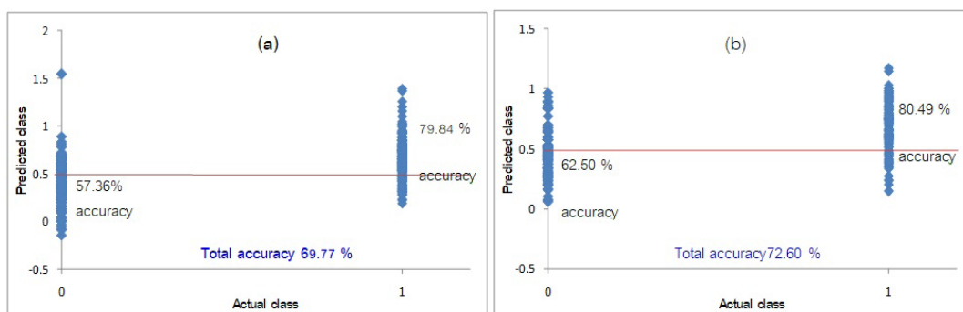
Figure3 Scatter plots of actual and NIR predicted values for rose apple fruit without eggs (0) and with egg (1) of fruit fly of calibration (a) and validation (b) group by MLRDA equation
