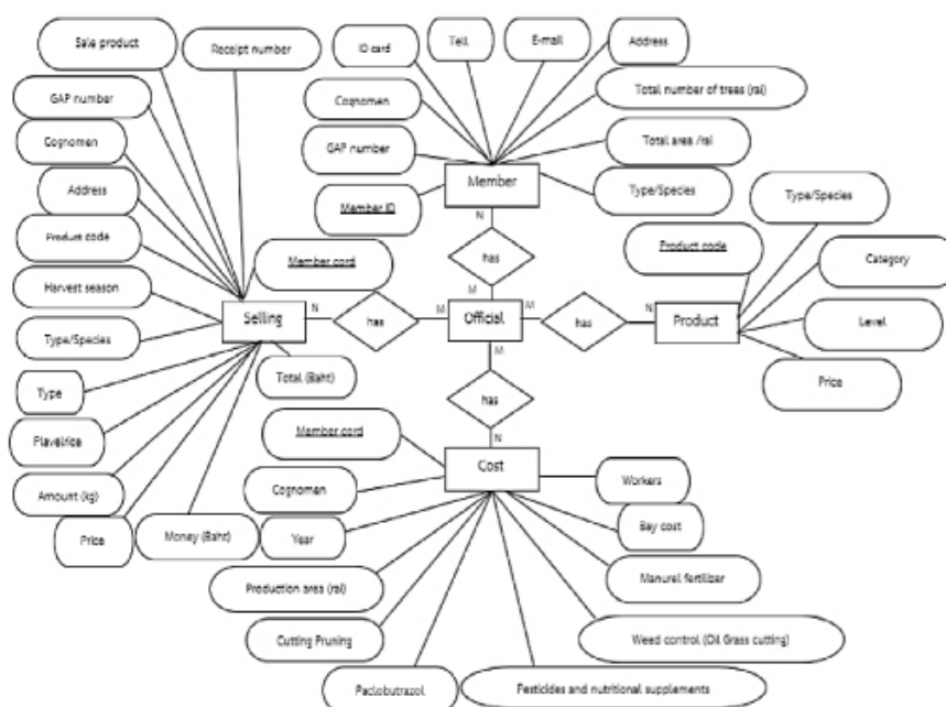
Figure 2 Entity relationship diagram: development of a cost-benefit analysis system mango for export
