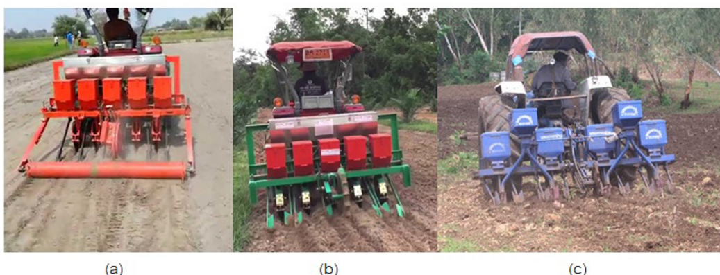
Figure 1 (a) Paddy seeder dry field connect roller embedding (b) Paddy seeder dry field embedding (c) Paddy seeder dry field 6 rows embedding
